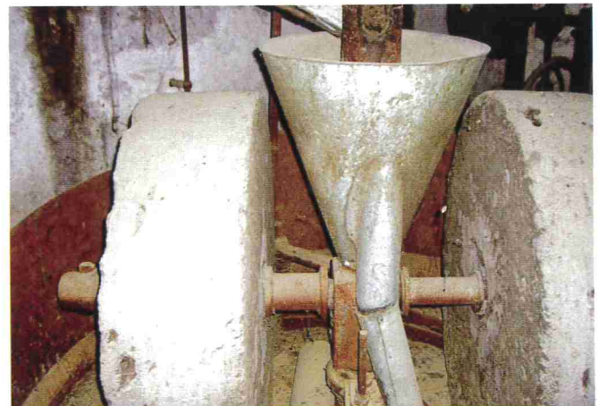
Figure 17 bis: meules verticales tournantes
